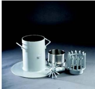
The M-170 measuring system is designed for testing of mortar and cement paste but works equally well with grout and cement based repair materials. Compared to the standard M-200 measuring system for mortar, that requires in excess of 12 litres of sample mix, the new M-170 measuring system now will make the test procedure more economical and less time consuming.
